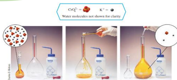
Gambar 61. Pengenceran Larutan K_2CrO_4 0,1 M Sumber: Whitten et al. , 2014
